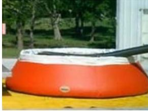
Upon arrival at the fire site, we will deploy a 500-gallon portable low-sided water tank with a floating rim as illustrated at left. It can be filled with seawater at a rate of 30-90GPM (subject to elevation). The presence of the tank will allow pumps carried in the 1<sup>st</sup> Response Trailer to draw from it and each lay water or foam on the fire at rates of 15 or 30GPM (as appropriate). This arrangement is designed for continuous operation.
